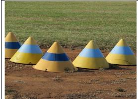
Cones that define the edge of a helicopter taxiway where a line marking is not present.
