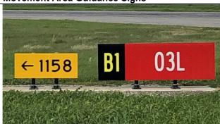
Parafield Airport has an extensive system of Movement Area Guidance (MAG) signs throughout the movement area. Drivers authorised to drive on the movement area must be familiar with these signs.
