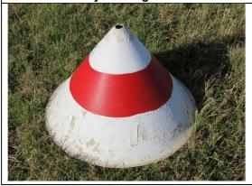
Unserviceability Cones designated areas of the movement area which are unserviceable or closed to aircraft operations. No vehicle may access the area without PAL staff approval.
