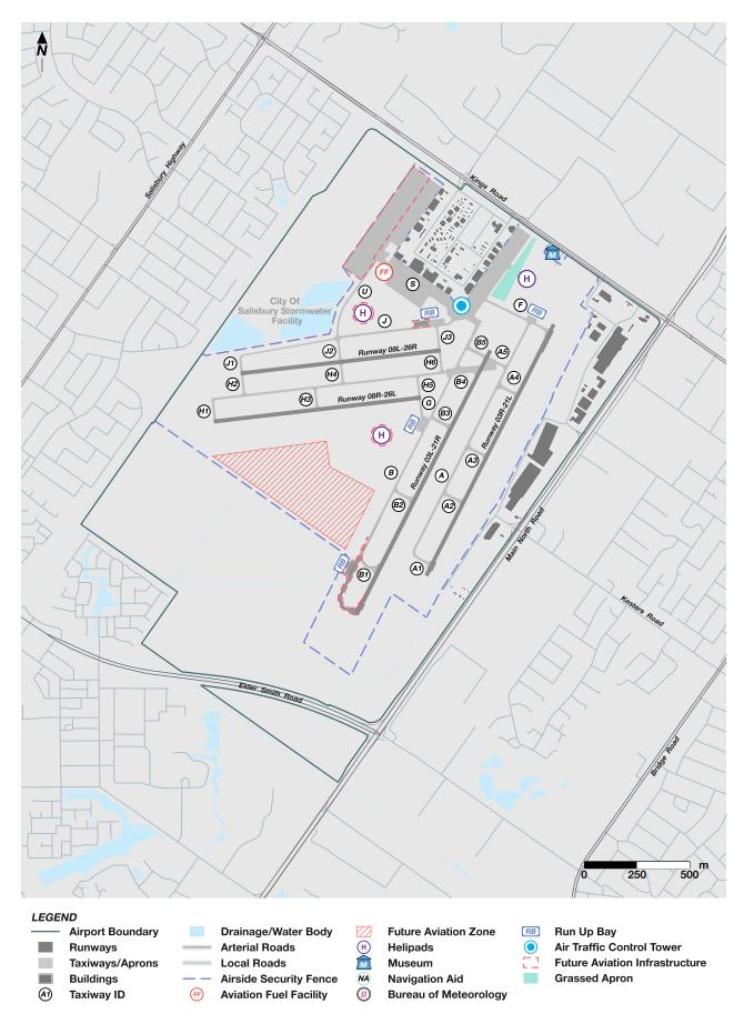
Figure 8.2: Planned airfield layout to 2043
